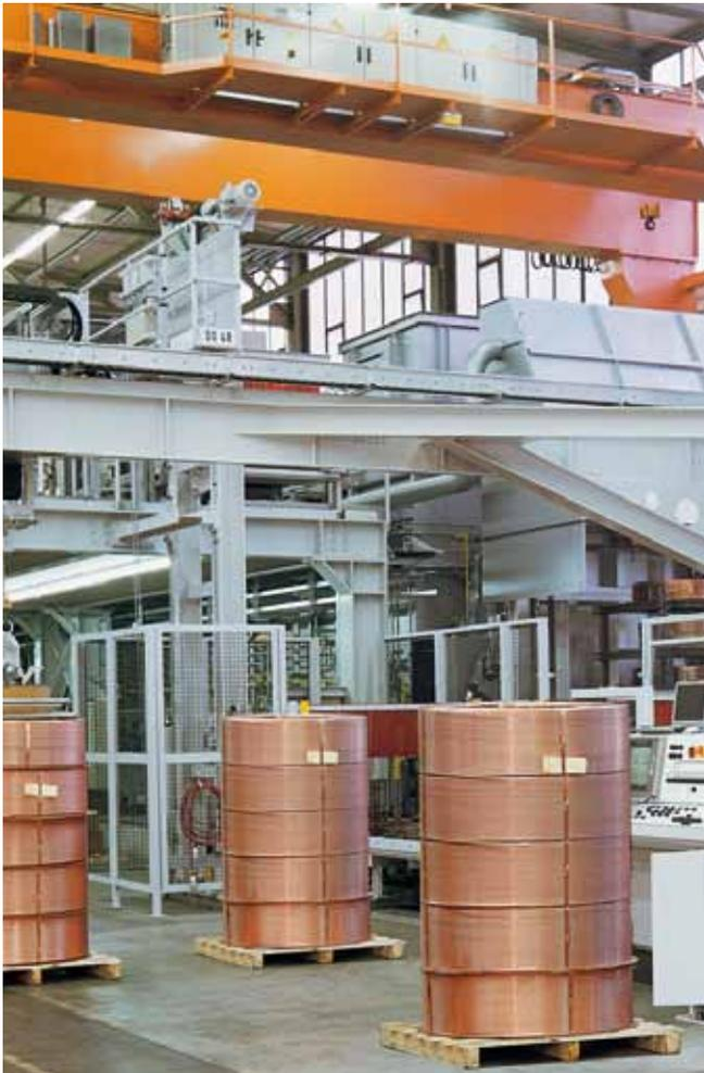
*Level-wound coils in copper (furnace behind)*
